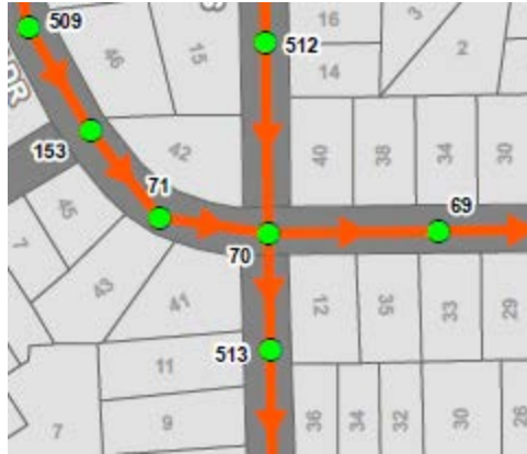
Figure 43: a problem occurs when four conduits intersect
