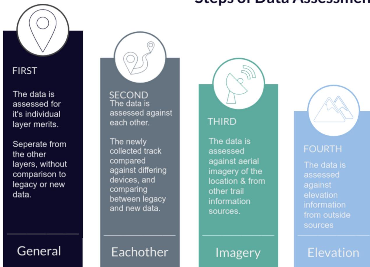
**Though this is done in steps for each trail individually, some of the process will happen simultaneously as the technician is scanning for inaccuracies, and errors; while flipping between elevation and imagery information.**
